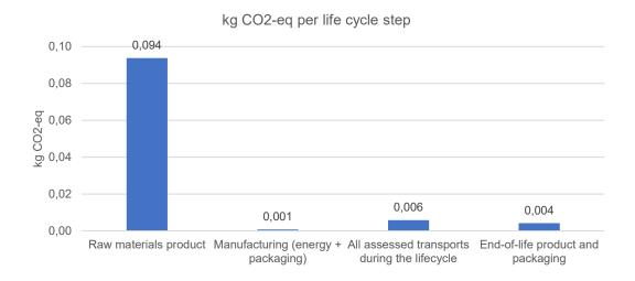
The raw material stands for the highest CO2-eq emission. The components that contributes the most to this result are the refill (tube and tip) and barrel.
